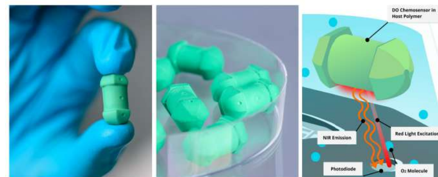
Sensor Pills Monitoring of CPPs like pH, Dissolved Oxygen, Glucose,...
